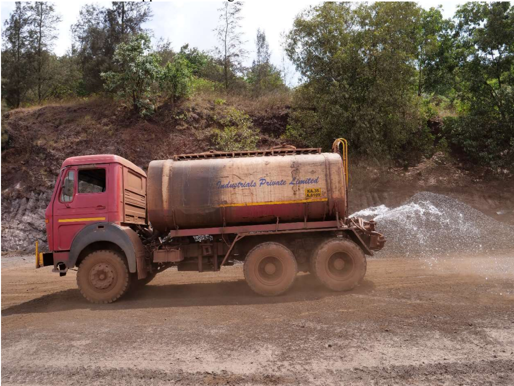
Dust Suppression on Haul road at Dabaxikolla-Governor Point
