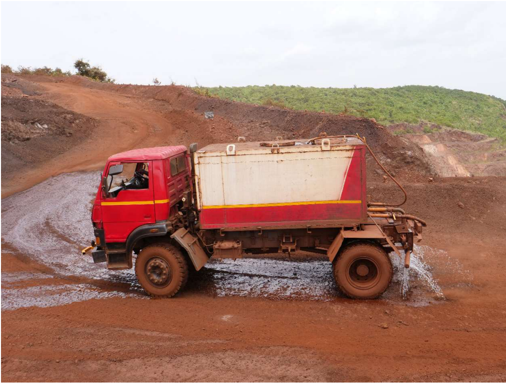
Dust Suppression at Neerlabbi Mine Pit
