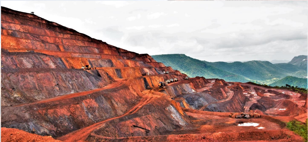
Scientifically and systematically developed benches Iron Ore Mine
